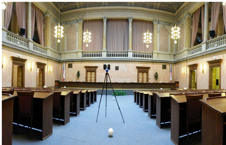
Photo of The Chamber of Deputies with FARO scanner and reference spheres
